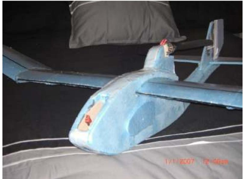
Check the leading edge and under the center of the wing; both reinforced with carbon. Even had a small piece left over so I hot glued it to the bottom, on the rear. (Think I may need an air scoop on the top to cool the ESC?)
