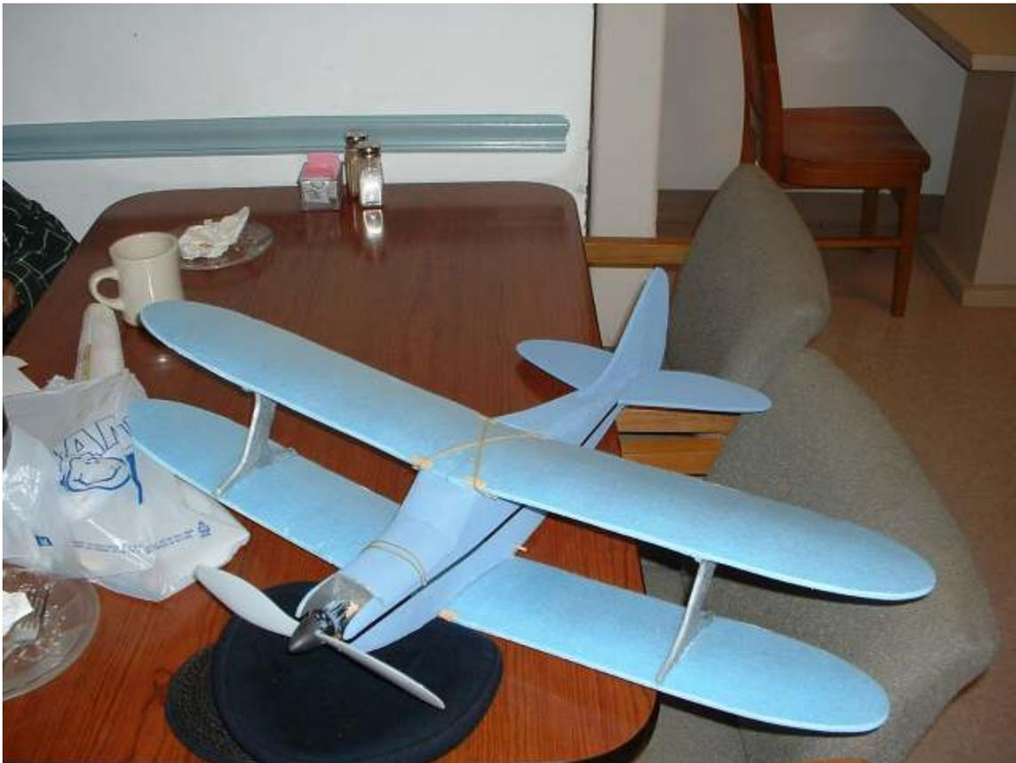
Weight came in around 14 oz. He uses a GWS twin drive. The model was painted with hobby acrylics for only a modest weight gain. He's flown the model and said it fly well. He will be experimenting with an aileron equipped model next. The plans for this model and others are available at:
